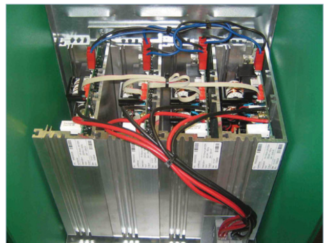
Parallel connected power modules, charger open
